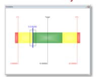
Uncertainty Chart added to display band around collected feature. This provides users a visual representation of how the gage performance affects measurement.
