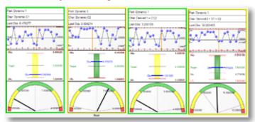
This function displays dynamic data from a data source at high sampling rates while providing a mechanism for discrete recording. Supports recording of Max/Min during capture and timed polling sampling. Two dynamic charts supported: Indicator bar and Meter chart
