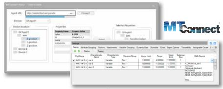
Agent data streams can be configured as Device channels. Inspection Routines allow mapping of characteristics to MTConnect Agent device channels as DAQ sources. All Real-Time functionality supported.
