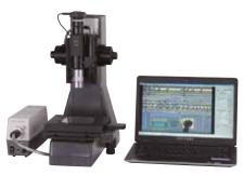
Digital microscopic system using VMU-V
