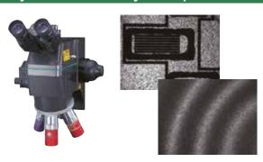
Optical systems using Mitutoyo M Plan Apo NIR objectives that cover a wide range of wavelength from visible to infrared are providing solutions on the production line and in the laboratory. Nondestructive inspection is made possible by using an infrared source.
